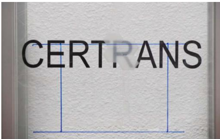
Figure 2: CERTRANS PROJEC. Pressureless sintering of magnesium aluminate spinel ( \text{MgAl}_2\text{O}_4 ) 3 ;
